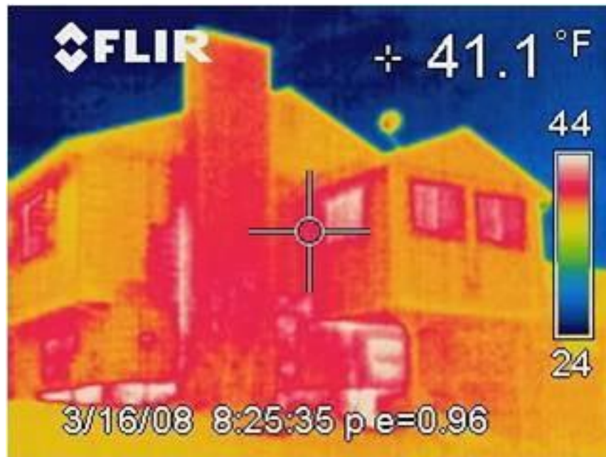
Heat leakage as shown by infrared camera, identifying where insulation and air sealing are needed. (source: DOER)
